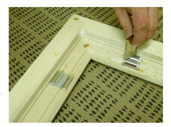
miter joints have been locate the rare earth magnets that the hardware package.
